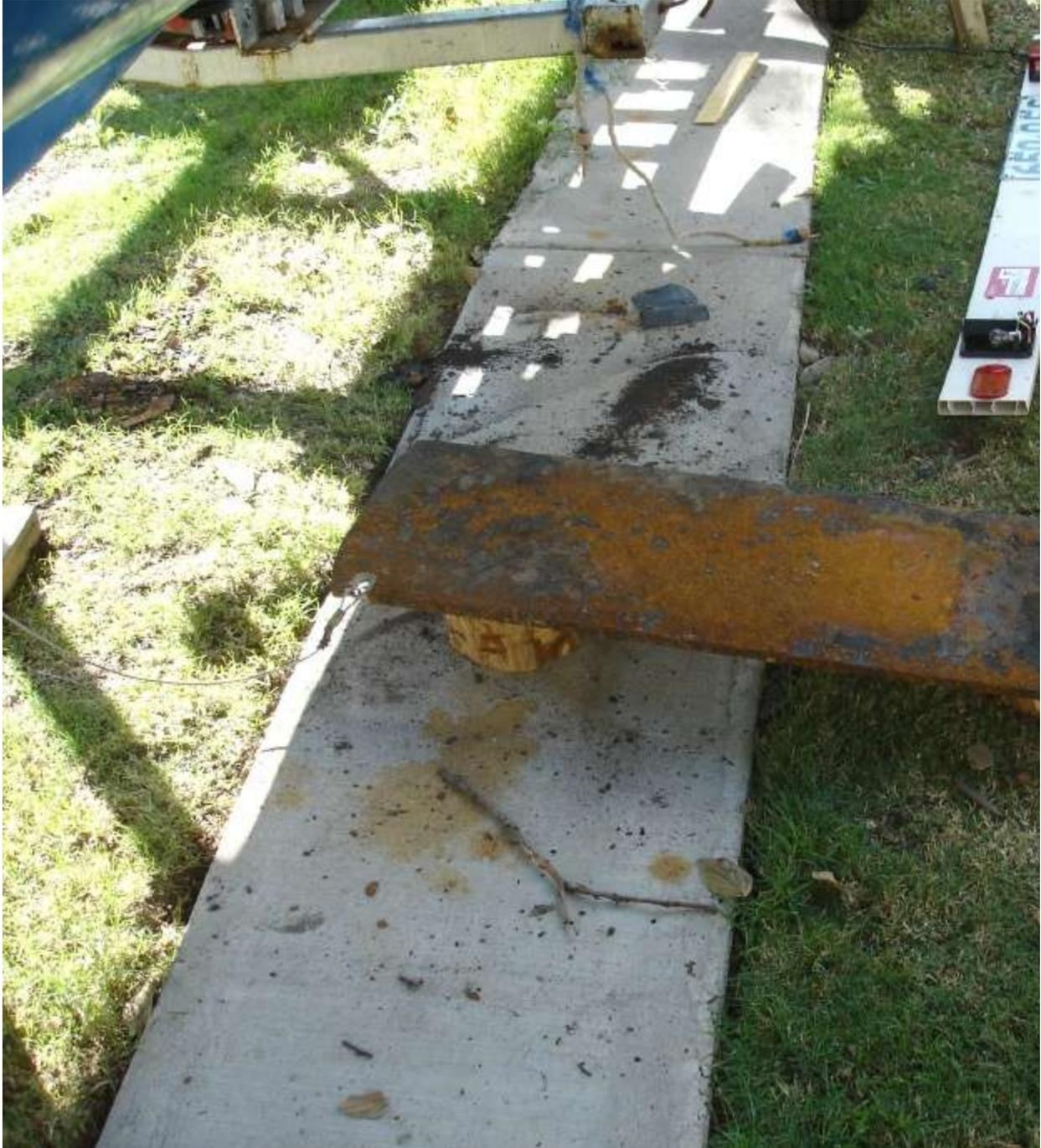
Then it was scraping off all the flakes and giving it a good banging, then wire brushing with a brush that fits the grinder. Then rust converter and finally cold gal.
